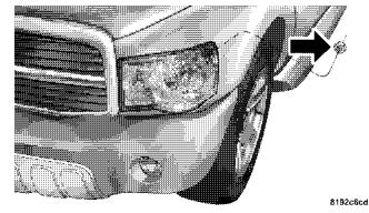
3. Grasp the headlight and pull firmly to disengage the headlight from the fender panel.
